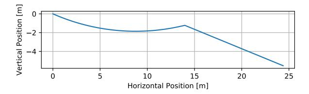
The takeoff angle of this jump was measured as 13 degrees. Using this angle the equivalent fall height can be visualized across the landing surface.
