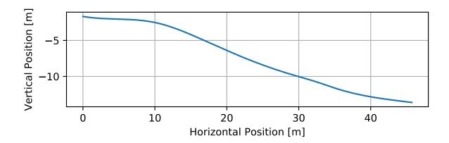
The takeoff angle of this jump was measured as 23 degrees. Using this angle the equivalent fall height can be visualized across the landing surface.
