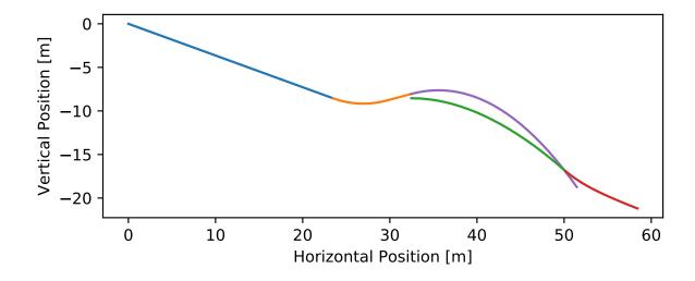
The design calculates a landing surface shape that produces a constant equivalent fall height. This can be verified using the <code>calculate\_efh()</code> function that calculates the equivalent fall height for the surface that was produced. See the <code>analyze jump</code> page to learn more about this function.
