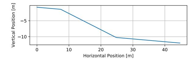
The takeoff angle of this jump was measured as 25 degrees. Using this angle the equivalent fall height can be visualized across the landing surface.
