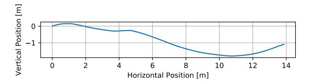
The takeoff angle is taken from the angle measurements. Using this angle the equivalent fall height can be visualized across the landing surface.
